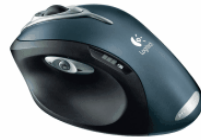
Figure 3: Interpreting differences in image fingerprints can be translated to movement of the mouse
